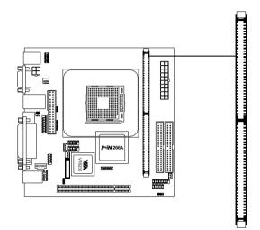
You can install either single sided or double sided 184-pin DDR DIMM modules into the DDR DIMM sockets, depending on your requirements. Differing from SDR DIMM, DDR DIMM modules have only one notch on the center of the module. The number of pins on either side of the breaks are also different. The memory modules will only fit if placed in the correct orientation.
