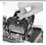
5. Connect the fan power cable from the mounted fan to the 3-pin fan power connector on the mainboard.
