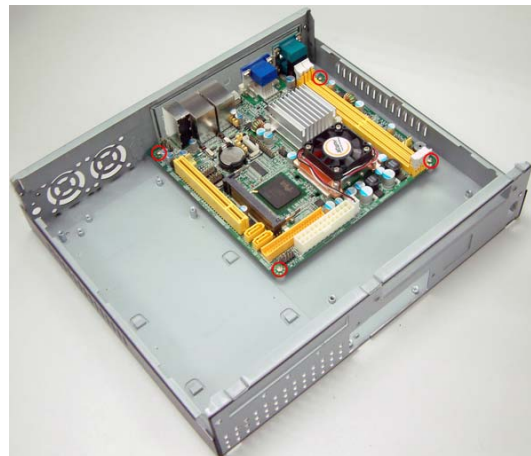
4. Make sure to fasten the screws through the motherboard to the pillars.
