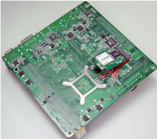
3. Plug in the Mini-PCI Express Interface Card at the angle of 45-degree.
