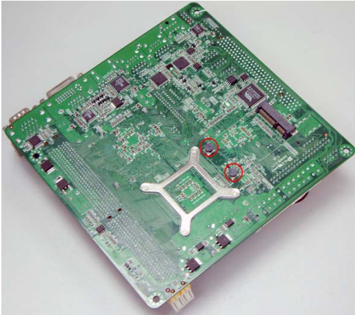
1. Loose two screws in the two rivets.
