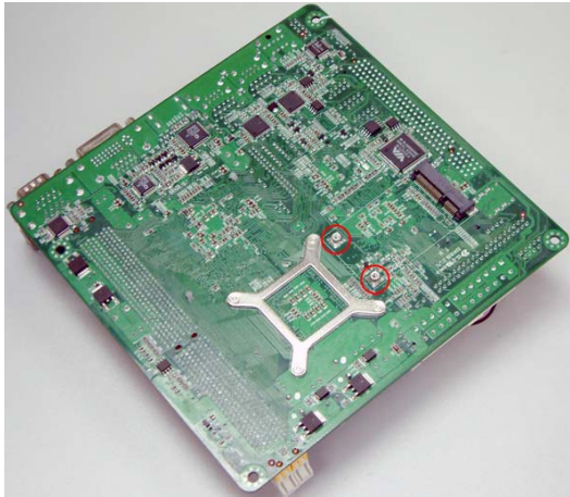
2. Ready to fasten the screws after installed Mini-PCI Express x1 compatible card.
