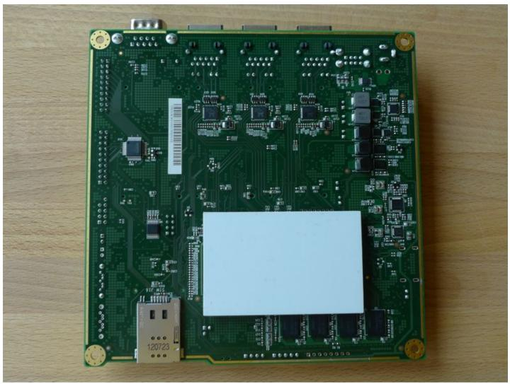
"Bottoms up" - hold the enclosure base upside down, feed the board DB9 and LAN connectors through the openings. Lightly press board and enclosure base together to stick the heat spreader in place.
