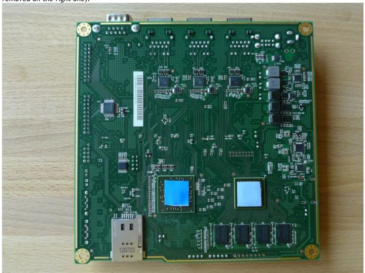
Place the alu heat spreader (blank side down) over CPU and south bridge. Make sure to avoid conflict with nearby through hole components. Peel the cover foil.
