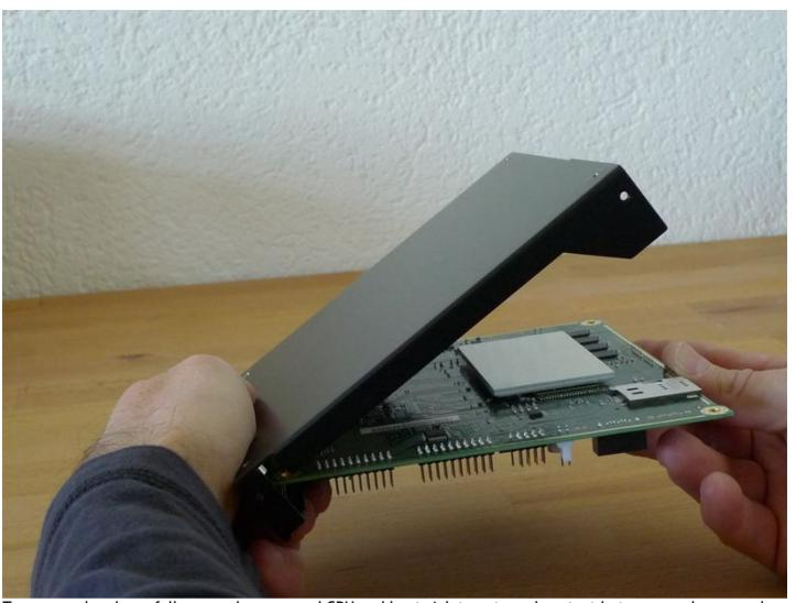
Turn around and carefully press down around CPU and heat sink to get good contact between enclosure and heat spreader. Then insert screws and hex nuts.
