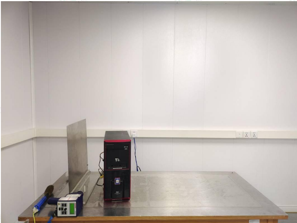
Test Setup Photo of Electrostatic Discharge Test
