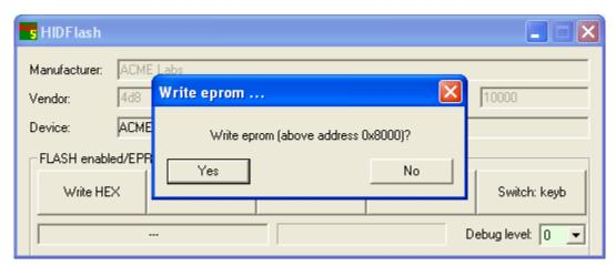
situated below address 0x8000. For the splash screen content the answer is "Yes", because the EEPROM memory field in the main controller is mapped on addresses above 0x8000).
