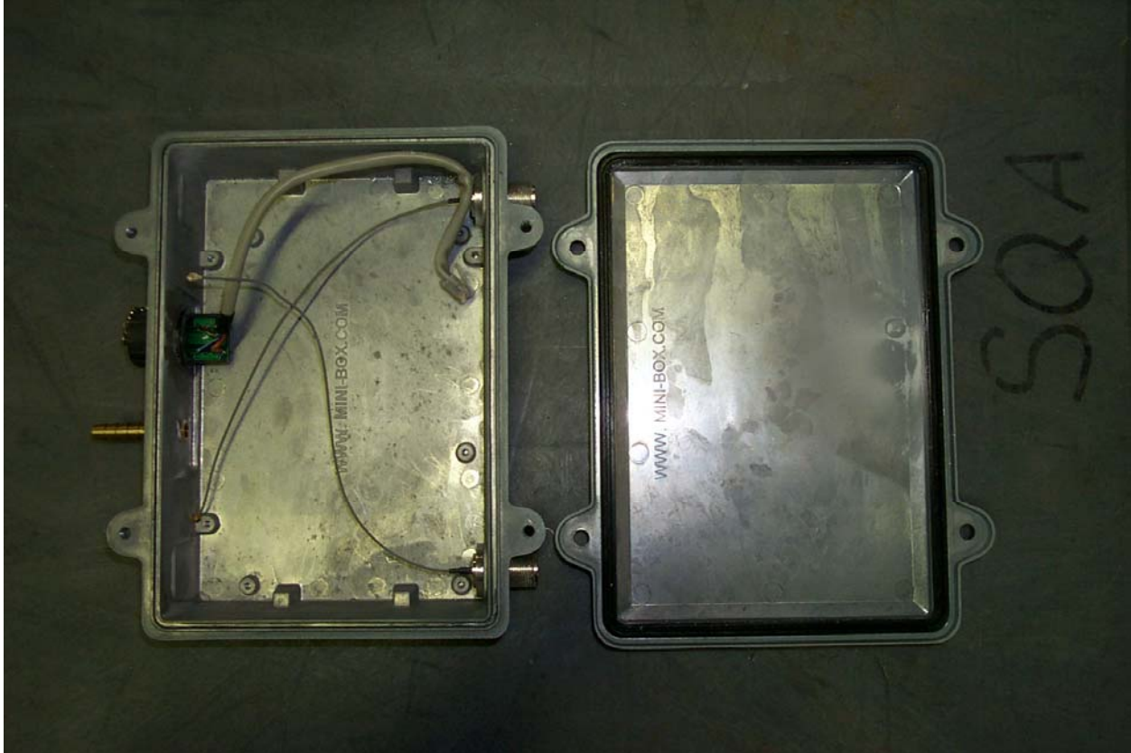
This is the interior of one of the enclosure after the Dust Test
