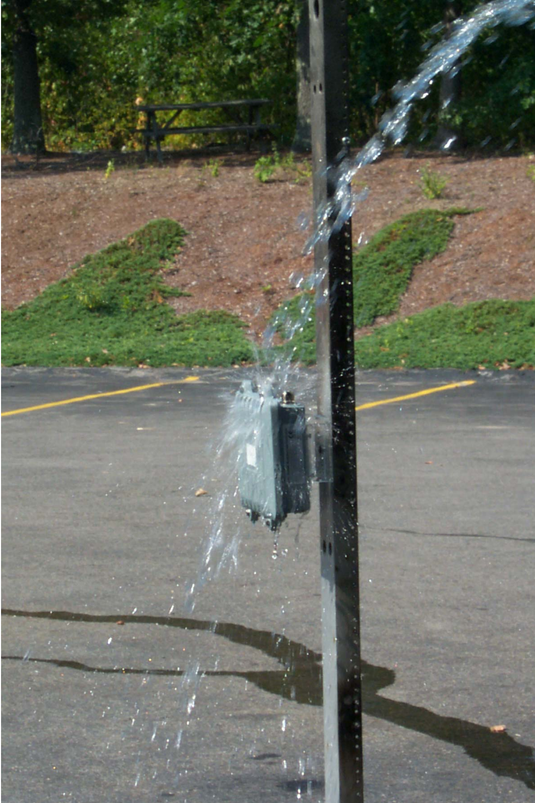
This is one of the enclosures during the Water Jet Spray Test
