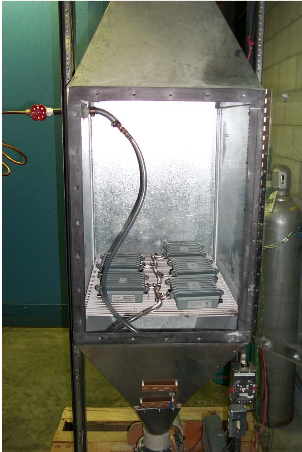
This is the Dust Chamber as configured for testing. The line coming out of the chamber is hooked to the vacuum.
