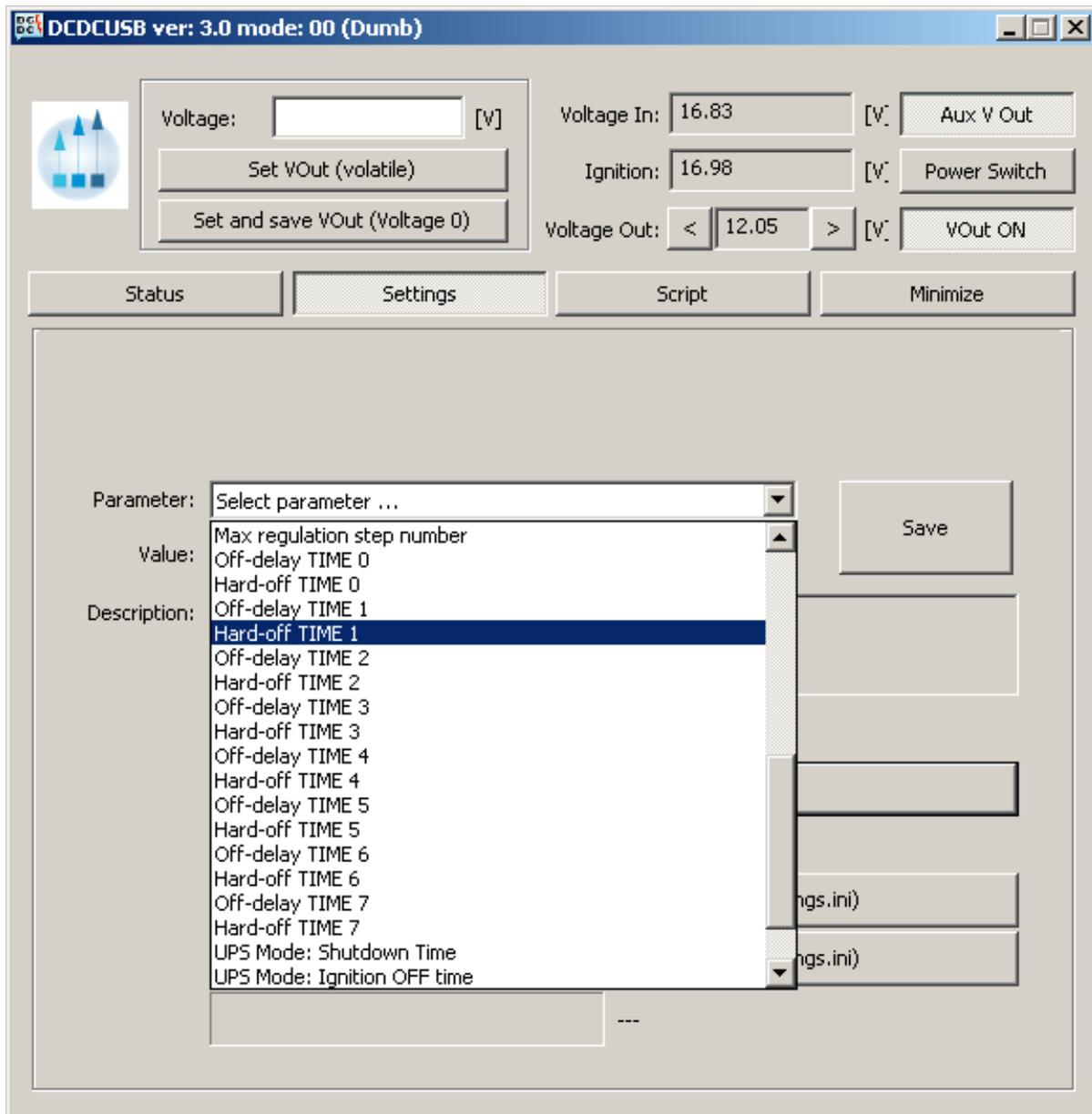
In this page you can see how several parameters can be configured by selecting it from the combo-box. After changing the value press the “Send” button to send it to the device. The parameter changed will have effect on the next power cycle.
