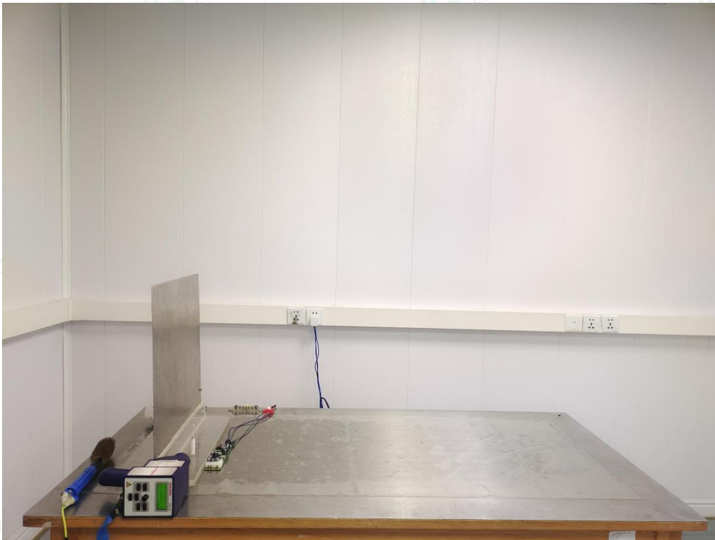
Test Setup Photo of Electrostatic Discharge Test
