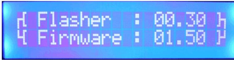
As you can see next to the displayed “Firmware:” text appears the firmware version number: “01.50”. In this moment the USB-LCD-20x2 device has a valid firmware in his main program memory and now is ready for use.
